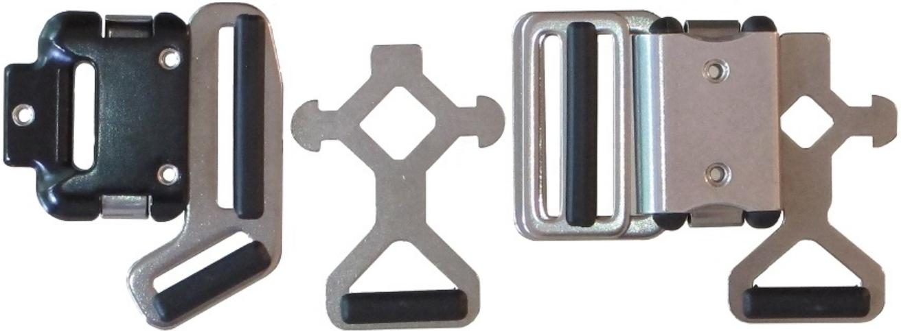
In the past three months, there have been two incidents involving older paraglider harnesses equipped with CLICK-LOCK buckles (HSi10) in the chest strap. The buckles had opened unintentionally during flight while they were under load. In one of the cases this happened during a SAT maneuver (spreading of the chest strap due to the pilot resting on the riser), in the other case the reason was presumably the load applied by the body weight of the pilot who was hanging only in the leg straps.
