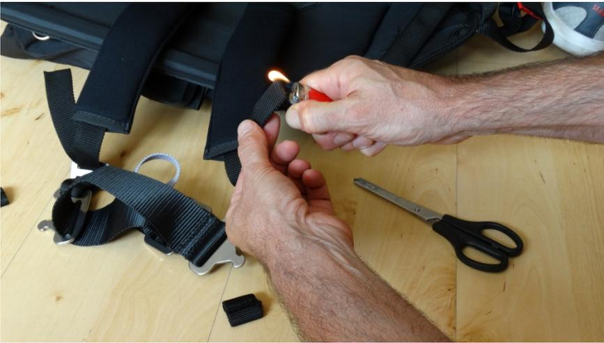
Burning the edges is to prevent the webbing from fraying and it can be done with a lighter or any other safe flame. Once the burnt edge gets cold again, make sure it is intact and does not fray.
