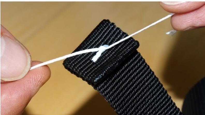
Make sure the chest strap is put together exactly as your old one by comparing it with the picture you took at stage #2 of the procedure. Now sew the blocking stitches on the ends of the leg straps as shown in the picture. Bend the final 1.5 centimeter end of the webbing over itself and sew it together with 5 stitched on one another using the provided thread and needle. Finally, make a knot and burn the loose ends of the thread away.
