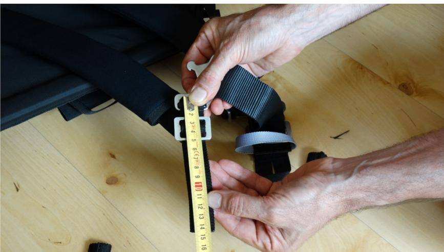
Before taking the chest strap off the leg straps, we recommend you to measure the leg strap adjustment as shown in the picture. Eventually, you will need this measurement to restore your harness setting.
