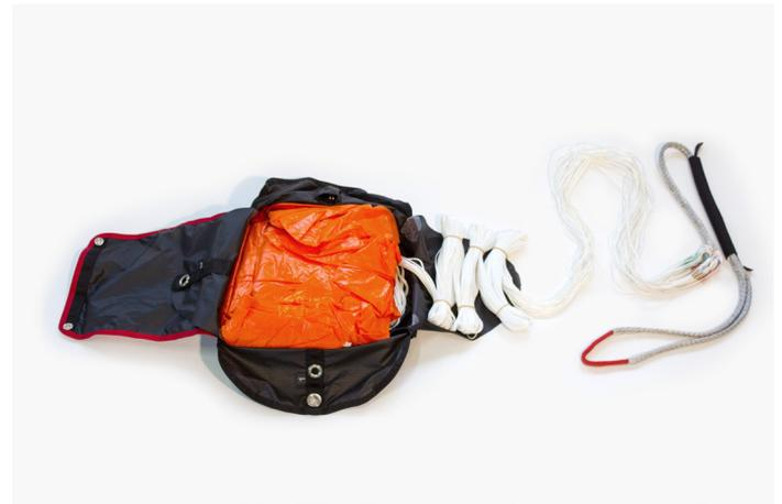
Close the container flap in the order indicated (1-3). Secure the final container flap (3) with a 5 to 6 cm line loop (ca. 3 finger widths). Now check the tension of the bungee loop and adjust if necessary. --> lift the package by the lines - the weight of the reserve should release the line loop.
